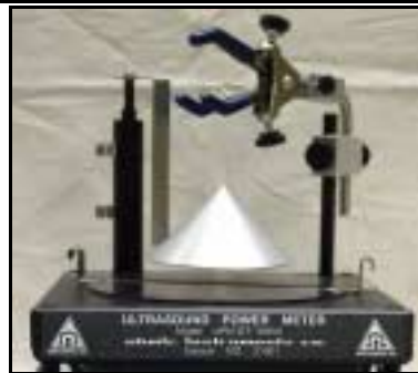
The cone target and transducer positioner. Tank not shown
